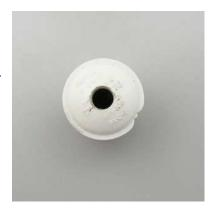
2. Insert one or two rubber washers (O rings) inside the coupler (depending on its depth).
