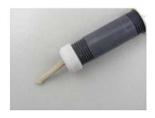
There are several advantages to this self-made clay extruder – first of all, its low cost. Also, each part is easily and cheaply replaceable. Anything that touches the clay is made out of plastic, so there will be no unwanted chemical reaction with the clay. And last, since a coupler is used, all icing tips can be used as well, which opens up a whole range of decorating possibilities.
