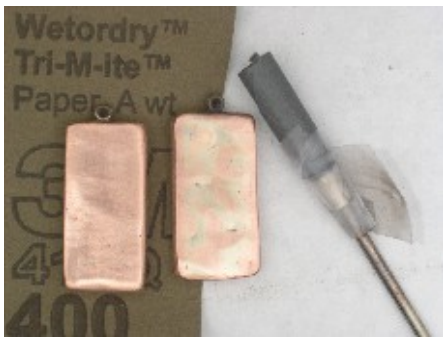
Sanding with 400-grit sandpaper mounted on a straight head slotted mandrel
