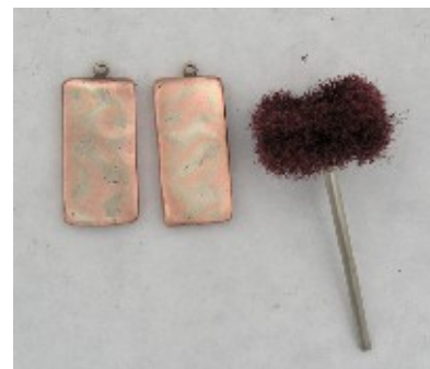
Sanding with 220-grit sandpaper mounted on a straight head slotted mandrel
