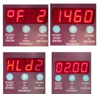
After pressing the left button again the controller displays °F2, which means the the temperature you would like the kiln to reach the second time around.
