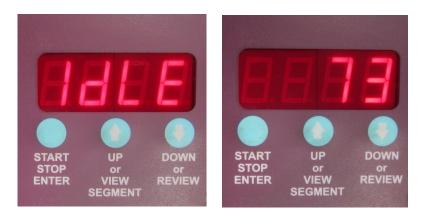
Before programming, the kiln alternately displays the message "IDLE" and the current room temperature (73 in this case).
