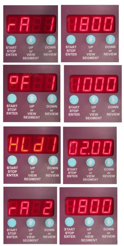
After pressing the left button again the controller displays rA1, which means the ramp speed you would like to start with.
