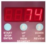
After pressing the left button again the controller displays room temperature, the temperature will start going up and you will hear the kiln clicking.
